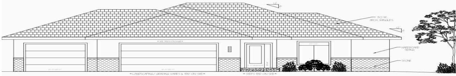
ELEVATION A: Front View - Roof Pitches Drawn at 6/12 & Overhangs Drawn @ 24".
